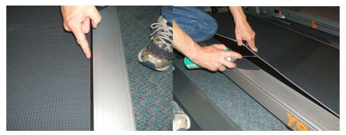
After spraying under each side of the mat with silicone spray, push with feet again to centralise the mat. Run the treadmill slowly checking mat is not rubbing against the siderails.
