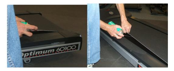
If the walking mat is covered by the siderails, push with feet to one side until the mat can be lifted. Apply silicone spray as above.
