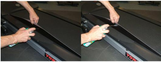
Lift up the mat and spray silicone spray onto the deck along each side, right into the middle and the complete length of the treadmill deck. For best performance and reliability ensure a good coating of silicone spray is applied to each side regularly.
